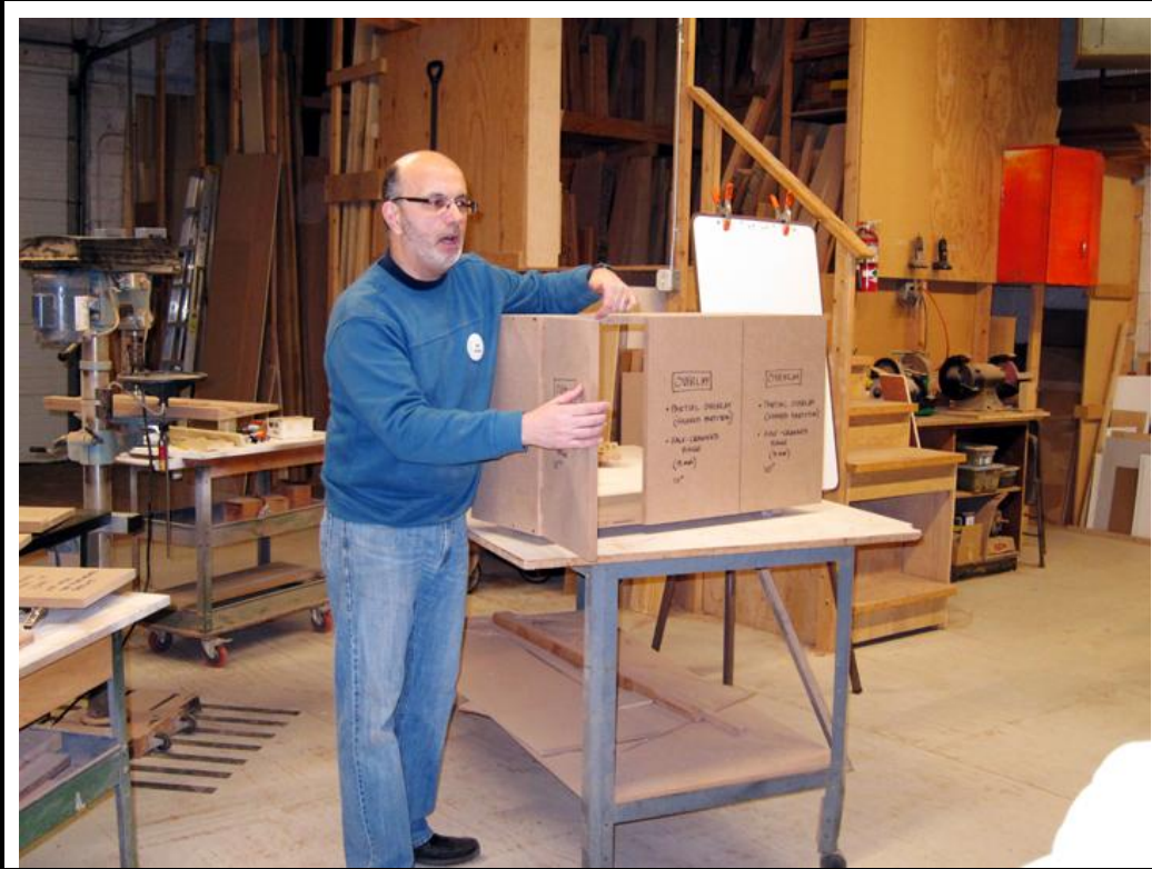
Bill shows how the hinges mount to the carcass and provide a significant amount of adjustment and flexibility
