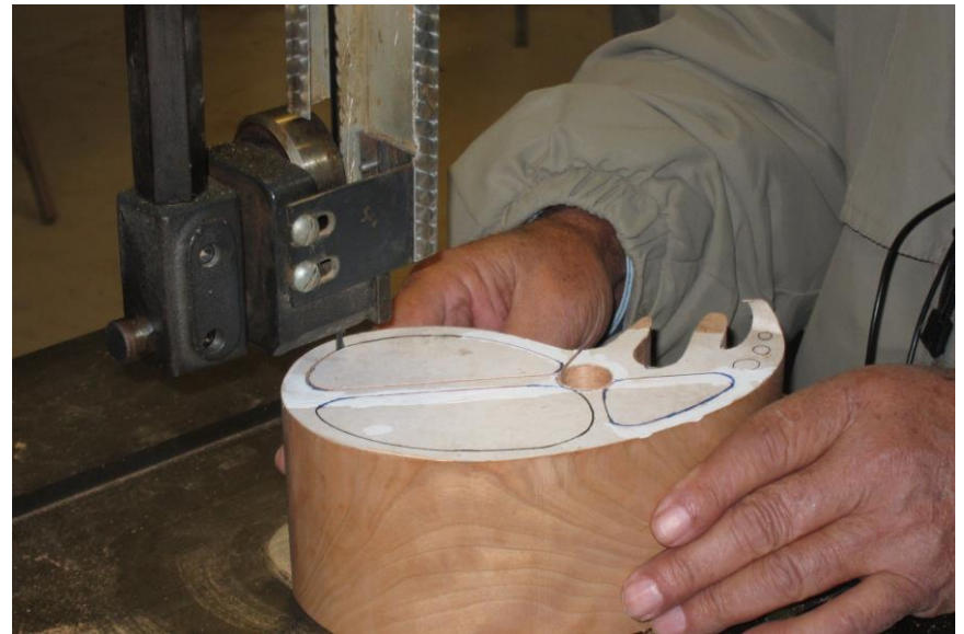
A paper pattern is adhered to the blank. Mohamad then saws out the blanks on the bandsaw
